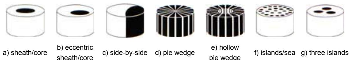
**Figure 2.** Typical bi-component fibre type.
