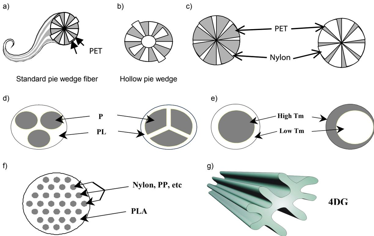
**Figure 5.** Schemes of fibre cross-sections with identification of the polymer used. The types presented in Figure 2 and 3 are given in brackets: a) standard pie wedge (Figure 2d), b) hollow pie wedge (Figure 2e), c) pie wedge with different polymer ratios (Figure 2d), d) three islands and three islands modified (Figure 2g), e) sheat/core and eccentric sheat/core (Figure 2a and 2b), f) islands/sea (Figure 2f), g) 4DG™ (Figure 3d).
