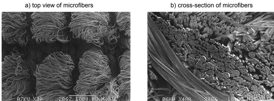
**Figure 6.** Scanning electron microscope images of microfibre cloth [21].
