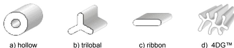
**Figure 3.** Typical microfibres with special cross-section shape [10,17,18].
