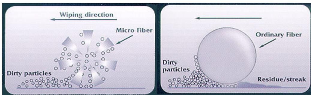
**Figure 7.** Scheme of cleaning dirt by common microfibres.
