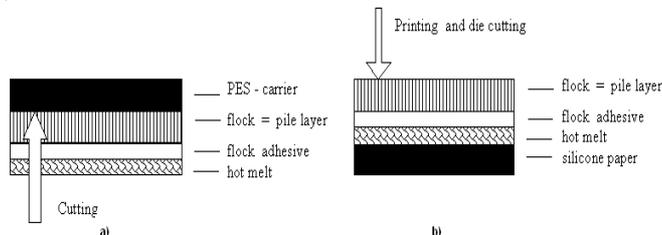
Figure 5. Typical structure of Flock: a) foil for cutting, b) foil for printing and cutting.
