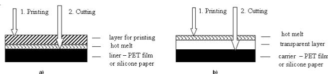
Figure 4. Flex-foil for printing a) typical, b) transparent - for print in reverse.
